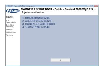
Example of calibration numbers entered in Delphi DDCR control unit on KWP2000 bus. For each injector is entered 16-digit calibration number, containing letters and digits.
