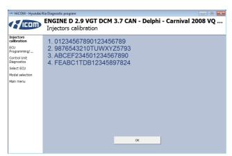
Example of calibration numbers entered in Delphi DCM control unit on CAN bus. For each injector is entered 20-digit calibration number, containing letters and digits.
