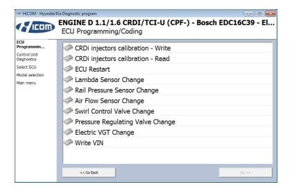
CRDi injector calibration is available in "ECU Programming/Coding" menu after connecting to diesel engine control unit.
