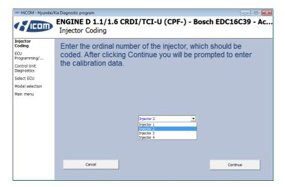
For calibration of new injectors, use "CRDi injector calibration – Write" function.
