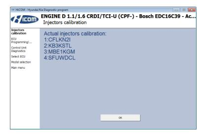
Current injector configuration can be read using "CRDi injector calibration – Read" function. This function is safe to use. It does not change any values.
