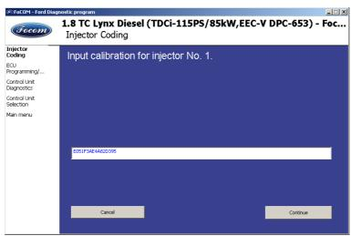
Enter calibration data of injector. Calibration data can be found on the injector or on the label placed in the engine compartment:
