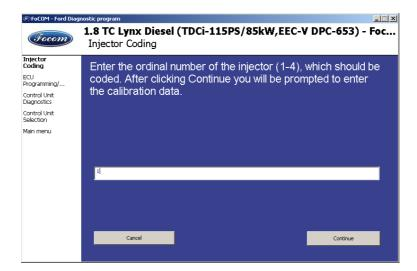
In the next step is necessary to enter calibration data for propriate injector.
