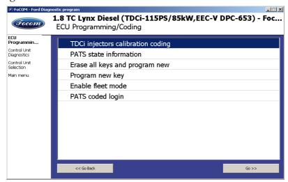
If you cannot find TDCi injectors calibration coding function in menu, please send us file with fast snapshot (go to the menu Control Unit Identification a click button Save ECU Information), part number of ECU (xxxx-12A650-xx) and the VIN code on address info@secons.com. A function will be added.
