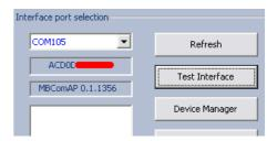
Now your computer is ready to connect to control units. In main menu, you can use either direct control unit selection (by clicking on *Select Control unit* button), or perform *Auto-scan*, which will list all control units installed in the vehicle. Make sure you have selected correct model and model year.
